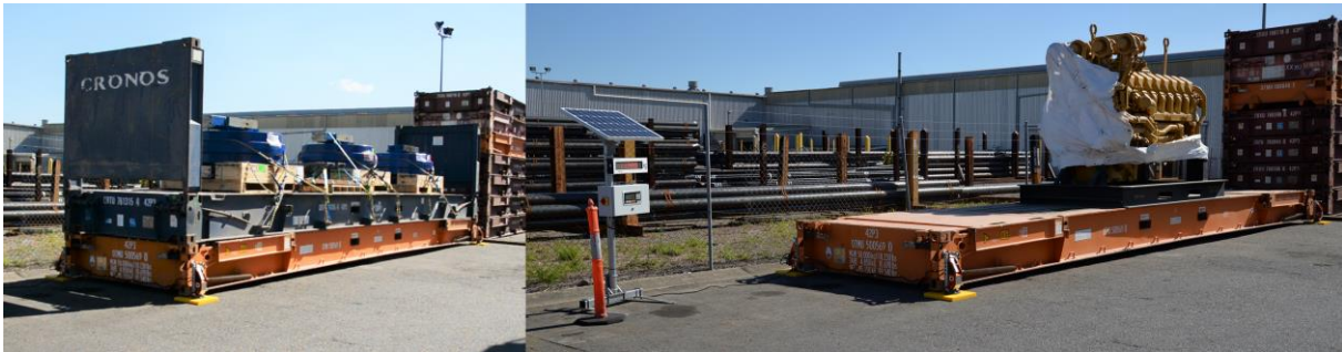
The Mobile Deck assembled from a platform container, weighing a loaded flat rack container (left) and machinery (right).
